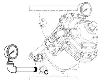
\*The pipe nipple is not required if the alarm test equipment is installed.
