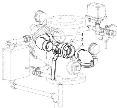
6.8 Inspection and drain connection
